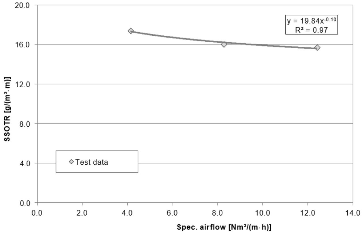
Figure 3-1: Results of specific oxygen transfer rate depending on the specific airflow rate per m of the air diffuser
