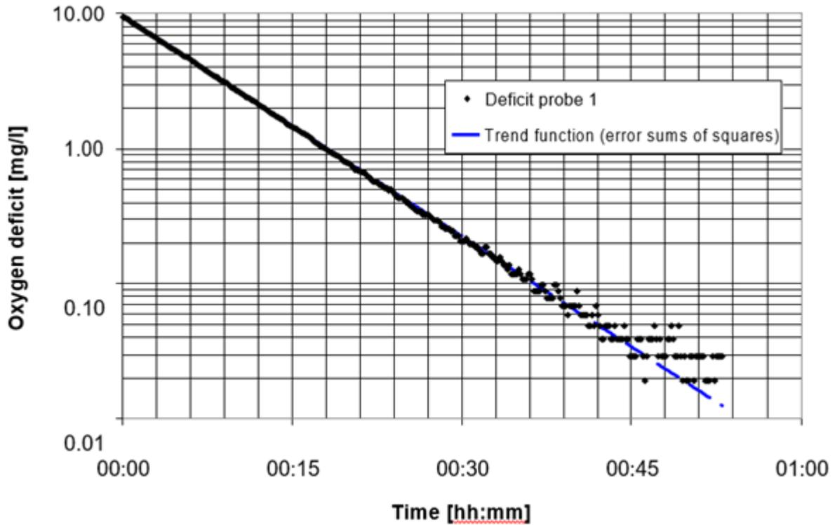
Figure 2-3: Oxygen deficit of the probe 1 on the measuring point 1 of the test with 16.0 Nm<sup>3</sup>/h
