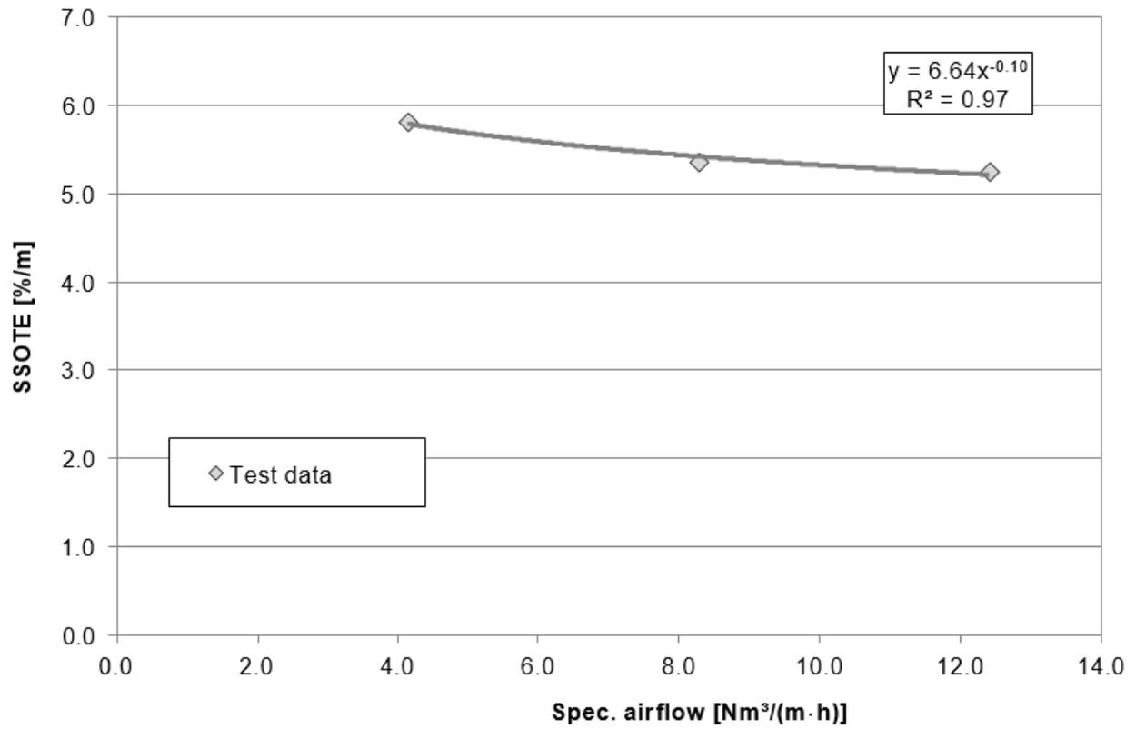
Figure 3-2: Results of specific oxygen transfer efficiency depending on the specific airflow rate per m of the air diffuser
