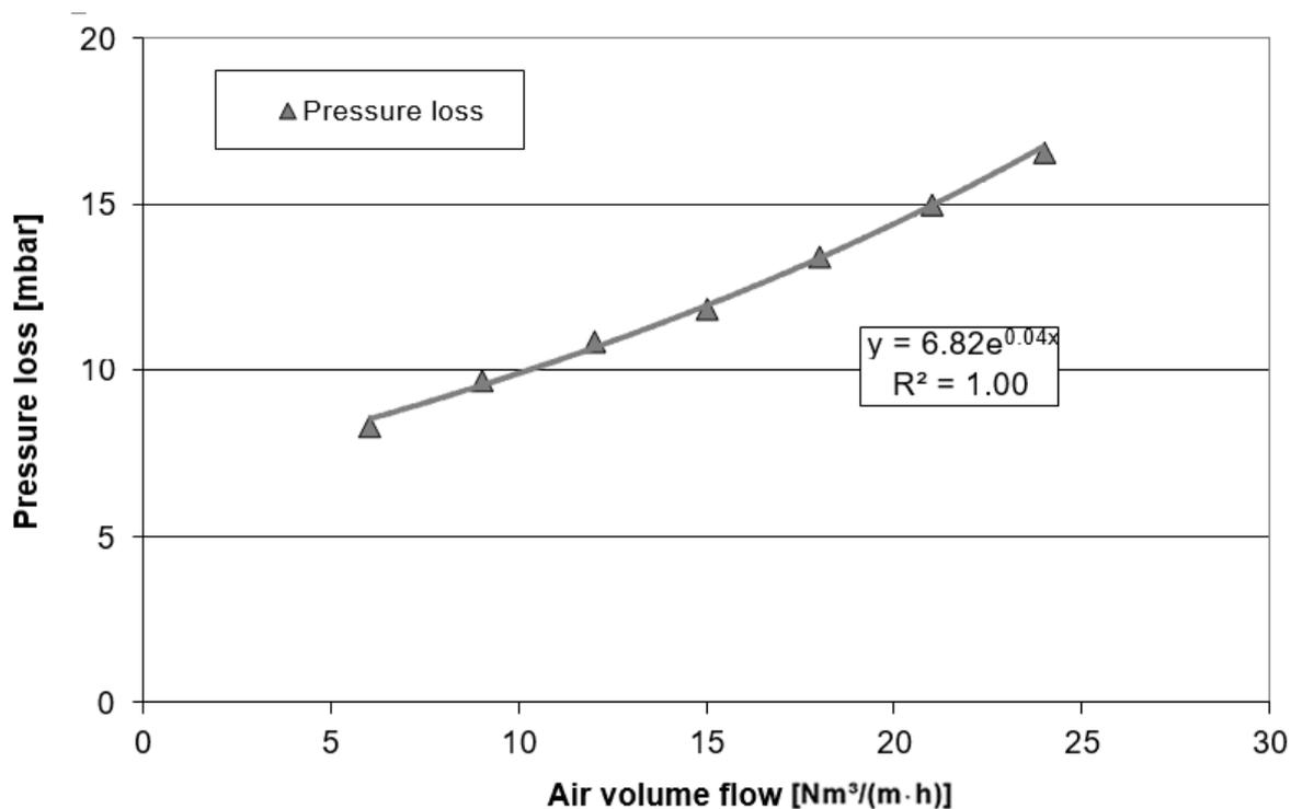
Figure 4-1: Results of the pressure loss depending on the specific airflow rate.
