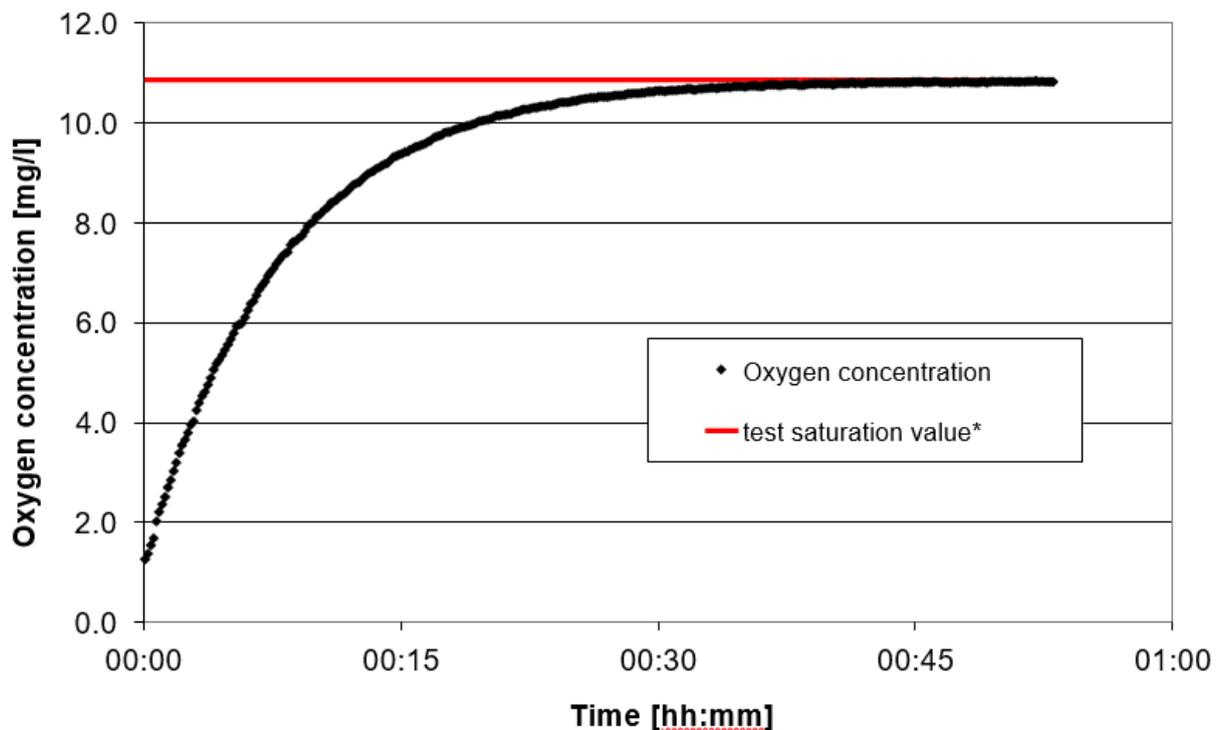
Figure 2-2: Oxygen concentration behavior of the probe 1 on the measuring point 1 of the test with 16.0 Nm<sup>3</sup>/h
