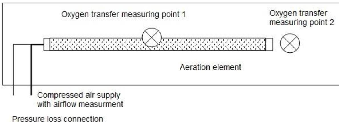
Figure 2-1: Test reactor with aeration element and measuring points for airflow, pressure and oxygen
