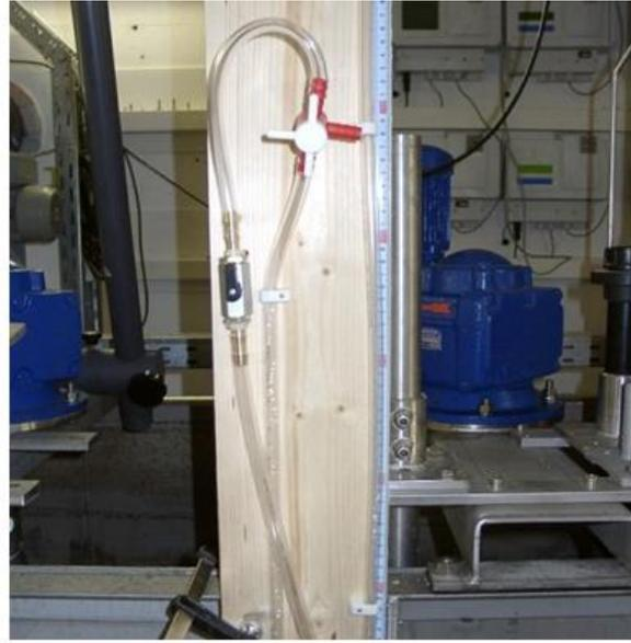
Figure 2-5: Schematic structure of the U-tube manometer and practical implementation
