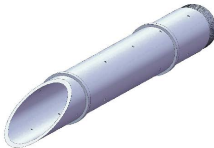
Figure 3.4 – Structure of aerator’s perforated framework.
