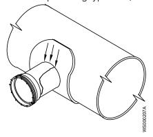
2. Chamfer the inside edge of the saddle opening to remove any saw cut projections.
